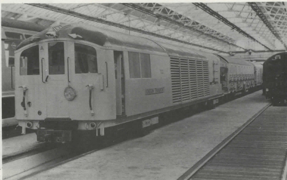
The Tunnel Cleaning Train TCC 1 to 5 at Ealing Common Depot 23-10-77. After many years development, this train has recently commenced tests between Acton Town and Northfields. (D. J. Burton)
