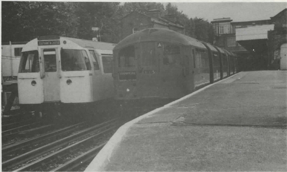
1972 MkII and 1938 tube stocks at Willesden Green during the first of the engineering works on the bridges at Kilburn on 18-9-77. The 1972 stock is seen on the Southbound Metropolitan track bound for Elephant and Castle, whilst the 1938 stock is on the Southbound Bakerloo track, working "wrong road" Northbound to Stanmore (B. Hardy)
