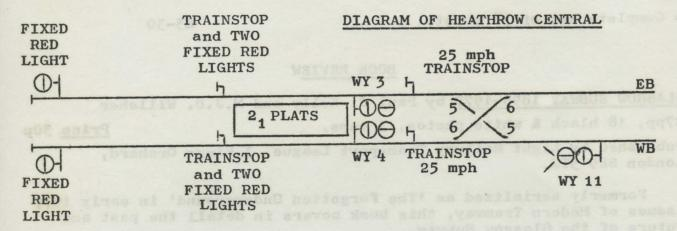
The two tunnels beyond the fixed red lights and trainstop (also fixed) are long enough to accommodate a train in each, but are not used as such, merely being over run tunnels. I believe that there are long term plans to extend the line further if another air terminal is built, to Heathrow West, Perry Oaks or even Staines has been suggested, and these over run tunnels would form the start of the extension.
