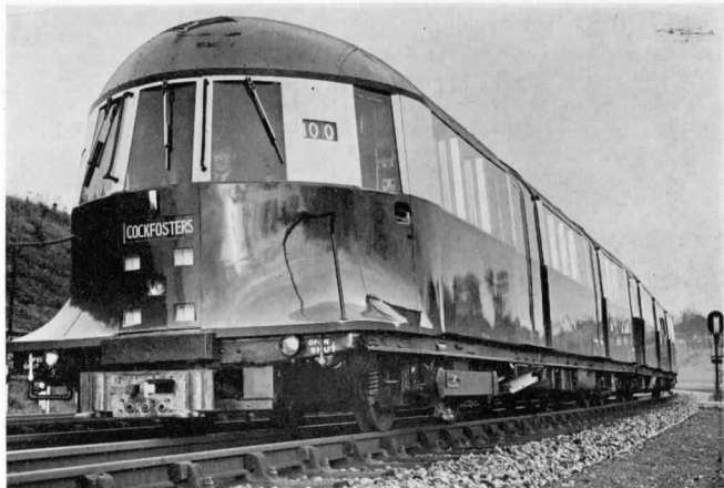
Car 10000 on the South Ealing test track posing for photographers, when new. Note the lack of opening windows on this unit which was the only one fitted with forced ventilation. [L.T.E.]
