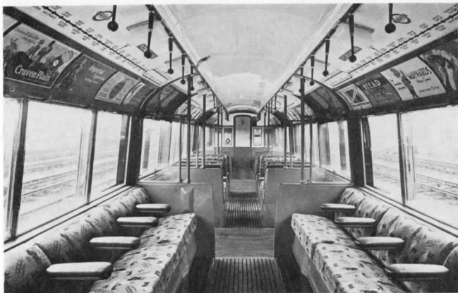
Interior of car 10000 when new. Note that the car line diagrams are "handed" in that they are appropriate to the direction of travel on each side of the car. This photograph also shows an early design of the ball-type handgrip. [L.T.E.]
