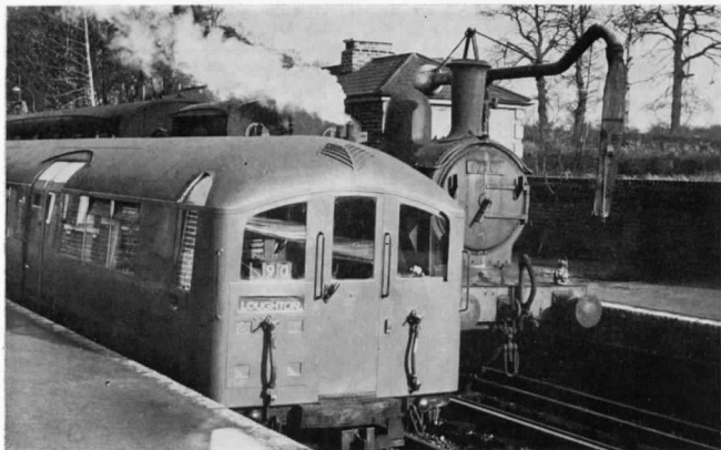
The West end of unit 10011-11011 at Epping, on the Loughton shuttle service, standing next to Worsdell ex-G.E.R. Class F5 (rebuilt from a Class F4) 2-4-2T No. 67202 on the Epping-Ongar push-pull shuttle. [Lens of Sutton
