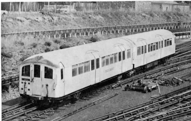
A view of 10011-11011 unit running into Northfields depot, 8th July 1971, on articulation tests. The two bodies mounted on one bogie in the centre can be clearly seen. Note also that the cars are substantially shorter than when new. [R. J. Greenaway
