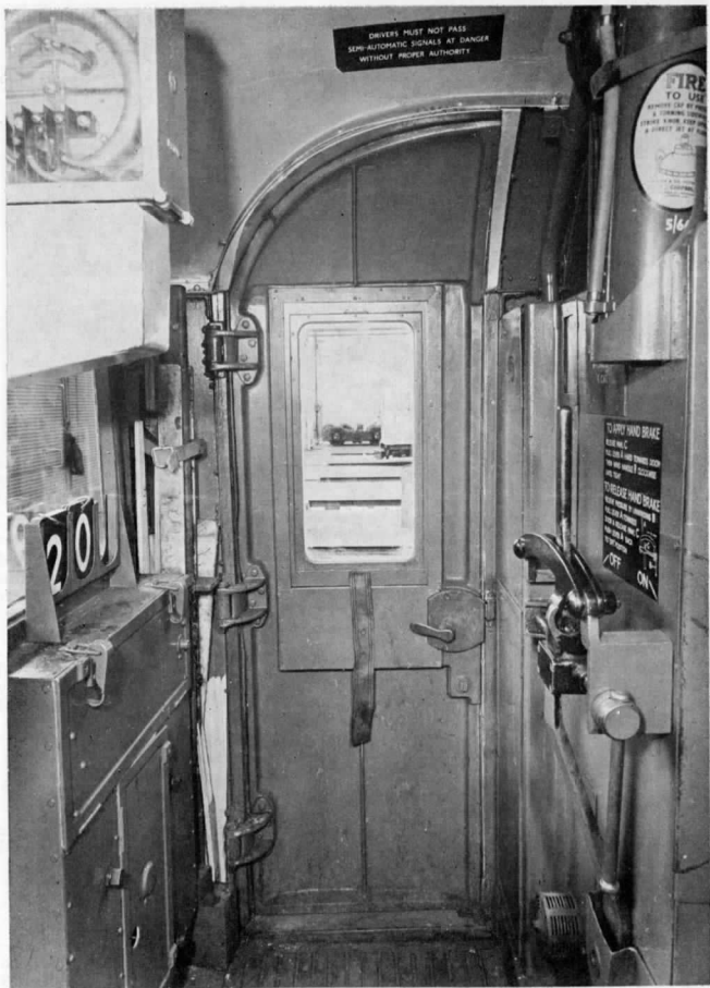
Interior of one of the flat-fronted driving cabs, showing that the cab door is hinged on the opposite side to 1938TS, and that it extends up into the curve of the roof. This was because, when new, the Guard's controls were fitted to the bulkhead (to the right) next to the handbrake. [L.T.E.]
