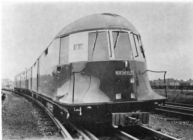
Car 10006 at Northfields depot when new. All 24 cars were delivered having positive shoe beams at the cab ends only. It should be noted that the front cab door extends slightly above cant rail level on this, and some of the other cars. [L.T.E.]
