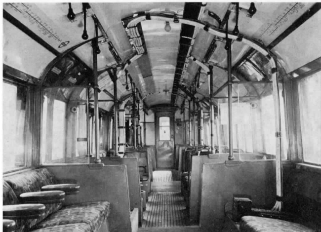
An interior view of 10011-11011 unit, equipped for regenerative braking tests in 1957, showing the wiring fitted inside the passenger saloon. Note that the line diagrams apply to the Piccadilly Line, being previously used on the Aldwych shuttle, and are above the advert frames, unlike the 1938 tube stock in later days. [L.T.E.]
