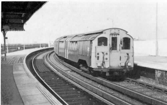
1928 U.C.C. car S19 working the pier shuttle. Note that the car no longer retains the curved side panels below the windows, and that this car is now withdrawn (see page 39). The curved platform at this station is well emphasised in this view, although the "Mind the gap" signs can only just be seen painted on the platform.
