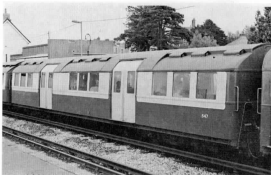
1923 Cammell Laird trailer in the latest livery on 7th August 1982. This type of car has side droplights, although with restricted opening, one of which is open on this car, S47. The fourth window in the centre bay has been blanked off where the luggage racks have been fitted.
