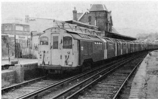
Spare driving motor car S10 coupled to unit 035 and another 3-car unit at Shanklin, 2nd June 1979. This car is the only one to retain its train number bracket which is used to indicate to which unit it is attached. Work on extending the down platform is in evidence on the left, while on the right can be seen the disused up platform. This has now been removed together with its track. [B. R. Hardy]
