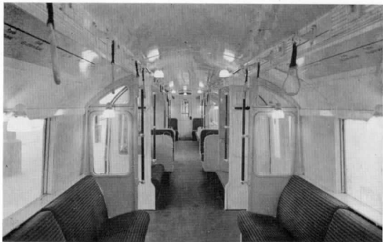
Interior of 1923 Cammell Laird trailer S47, 7th August 1982. This car has had its wooden floor lagging replaced with dark grey linoleum, its seating recovered in B.R. blue moquette, has lost its armrests, but retained the white handgrips.
