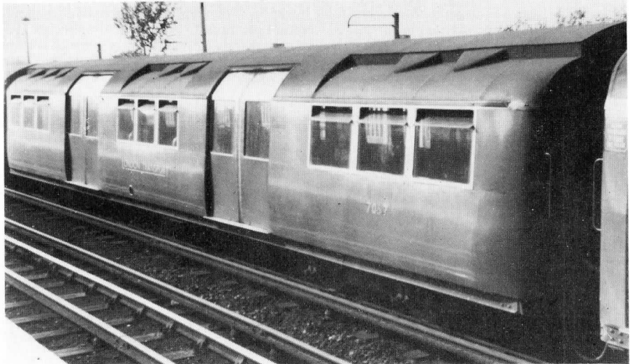
Above: Trailer 7057 of the 1930 UCC (Feltham) experimental train. This was one of two trailer cars with wider double doors than normal.
