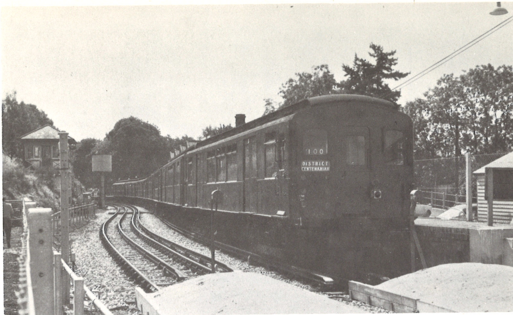
Above Q27 car 4357 at the head of an 8-car special train 'District Centenarian' at Chesham on 24-8-69. Q stock had briefly been used on the Metropolitan main line to assess the benefits of sliding doors on the line when eight Q23 driving motor cars were formed into a train around 1950, several having their motors cut out to limit what would otherwise have been a very powerful train.
