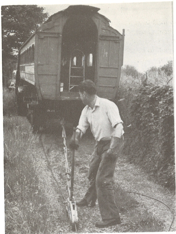
Top Paul Creswell taking his turn with the 'Tirfor' winch hauling the coach/chassis combination down the lane on 25-6-77.
