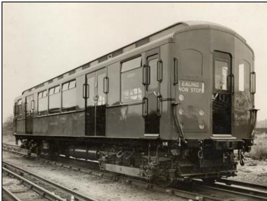
Fig. 1: Official photo of K Stock motor car as prepared for service in 1928. On the solebar, just forward of the cab door step, the letters “KM” appear. These apparently denote the stock identification code as K and the car as owned by the LMSR. However, this method of showing stock identity on the actual vehicles was inconsistent and appeared on some, but not all, new vehicles up to the 1937-built O Stock. Photo: LT Museum U5144.
