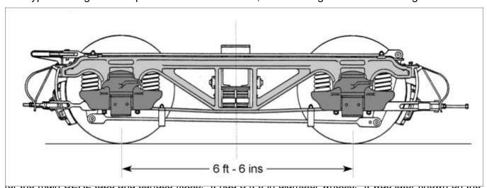
District as the Type A bogie. The frame was cast steel, then fashionable in the US but not in the UK. Cast steel is now the standard for most modern bogies. This drawing is a scanned and cleaned up version of one by the late Stuart Harris. My thanks to Andy Barr who dug out a set of Stuart's drawings and sent me a copy.
