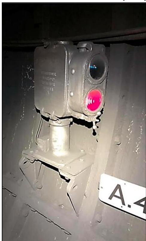
Figure 1: A colour light signal supplied by the Westinghouse Brake Company, confirming that it was designed before the formation of the McKenzie Holland & Westinghouse Power Signal Co. in 1907. This signal is believed to be located at Marylebone. Photo: Collection B.R. Hardy.
