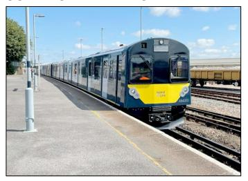
After intermittent night-time test trips, class 484.002 and 484.003 first ventured out in daylight test running on Tuesday 13 July 2021, seen at Eastleigh on a test run to Fareham.
