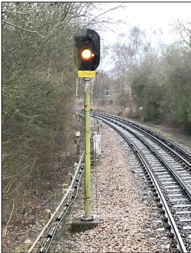
Figure 4: A distant colour light signal on the Chesham branch. This was a fixed yellow signal, with a ‘Distant’ label in yellow in place of an R number. There were two of these on the branch and they were unique to the branch. Photo: B.R. Hardy.
