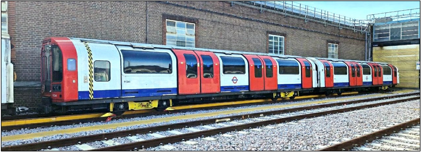
Above: 1992 Tube Stock unit 91341-92341 is a long term stopped unit in Ruislip Depot and is currently sitting on accommodation bogies.
