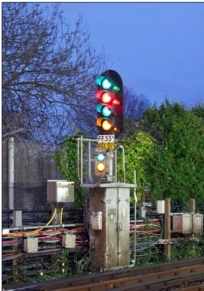
Above: ( Right ) A time exposure of the outer home signal at Upney eastbound, showing all possible aspects on the combined stop and repeater signal and also on the Fog Repeater below. All now history!
