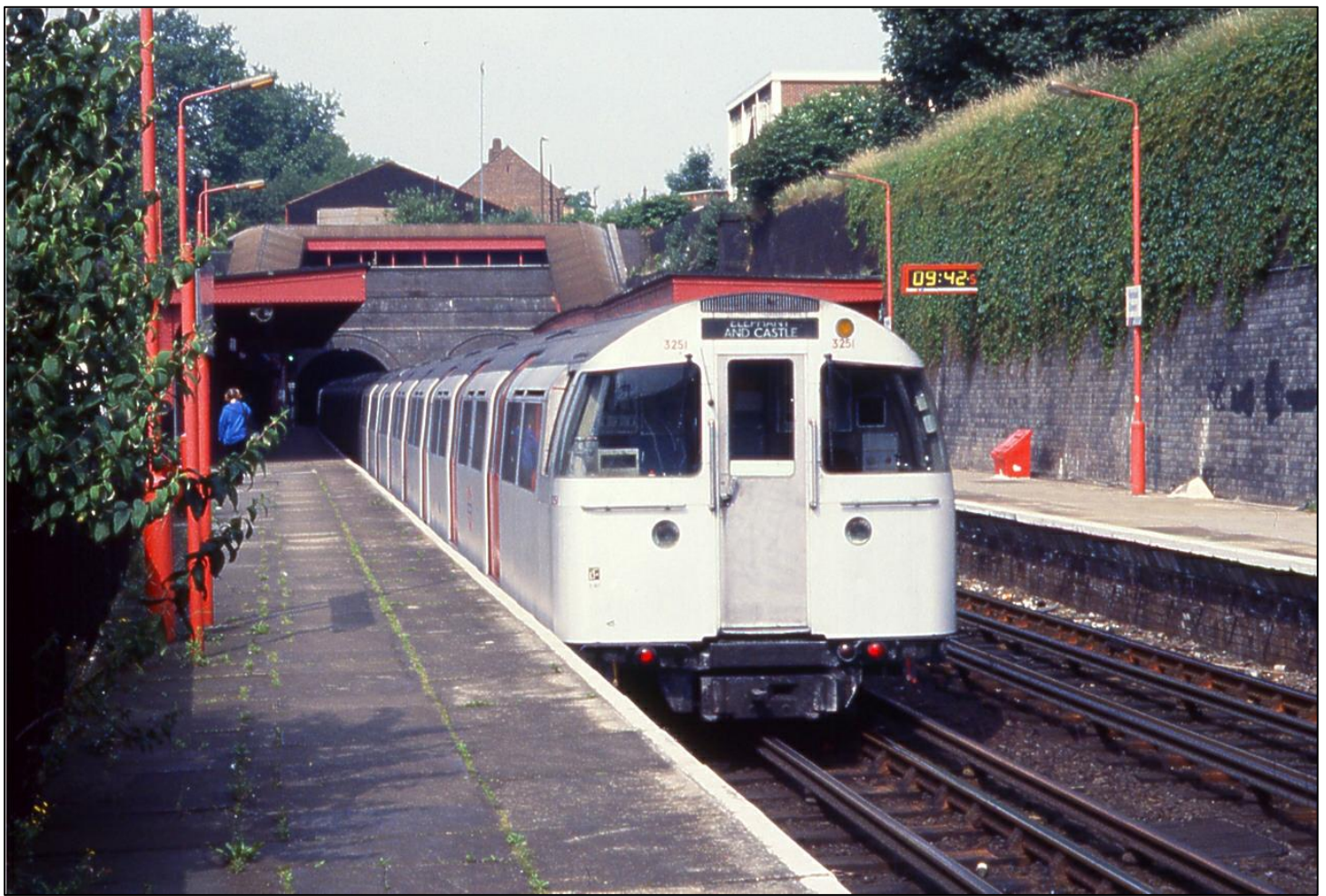
Above: When the 1972 MkII Tube Stock was converted to OPO, the train set number plates were replaced by an electronic display, which meant a change of set number could be done from either cab and display the same number at both ends. DM 3251 is seen at the rear of a northbound train departing from Kensal Green, bearing a Golders Green overhaul logo.
