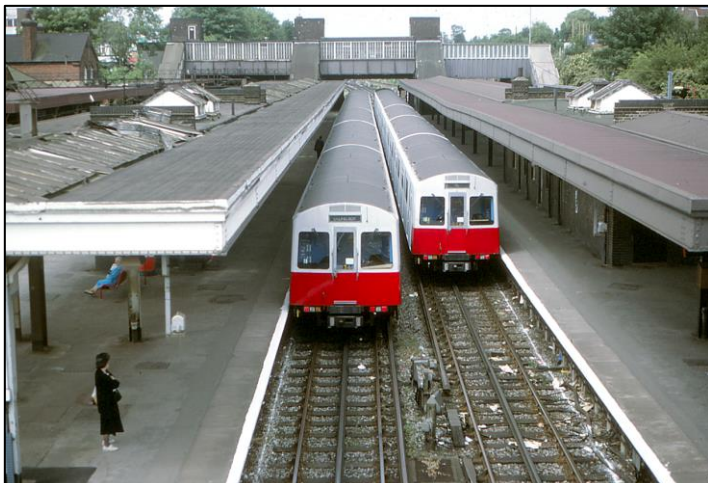
Below: Two D Stock trains side by side in platforms 3 and 4 at Upminster, the only notable alteration to the front end from new being the addition of a train radio aerial.
