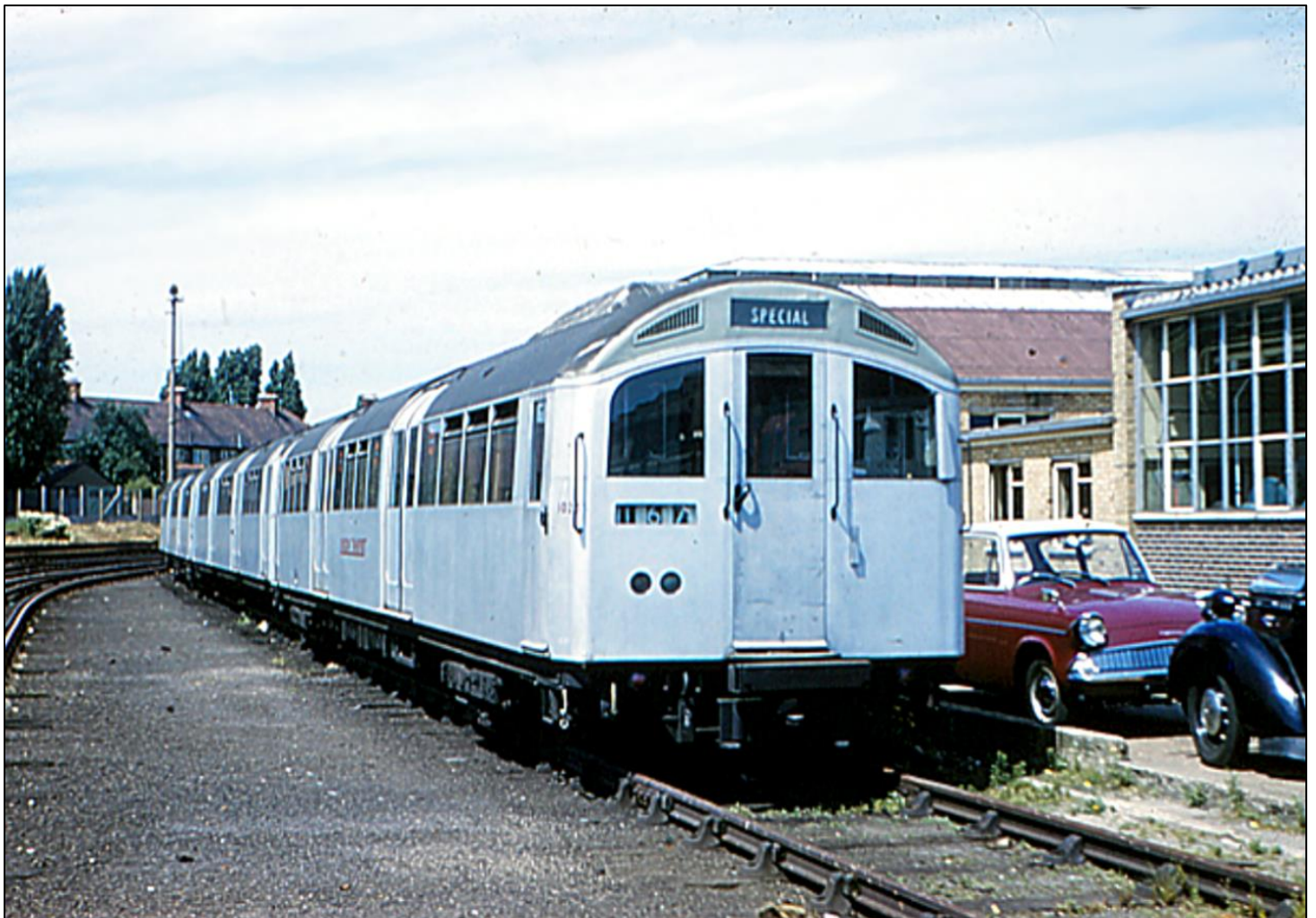
Opposite: (Lower): Awaiting its first overhaul is unit 1023-2022-1022 of 1959 Tube Stock in Acton Works on 20 July 1962. Its four-car partner unit (1020-2020-9021-1021) was also in at the same time, and being collision damaged, the whole seven cars were converted as a trial with electric door operation – it was known as the EDO train and 'EDO' was stencilled on the guard's panels as a reminder. At the
