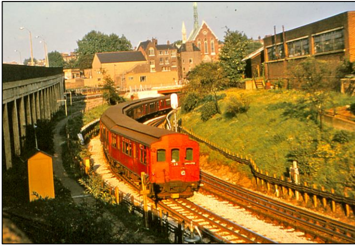
Above: An eight-car mixed Q Stock train departs West Kensington and heads for Earl's Court on 29 August 1962. Nearest is a Q23 former G Class motor car – a flared-sided Q38 can be seen towards the front. Access to Lillie Bridge Depot is under the Cromwell Road viaduct on the left.
