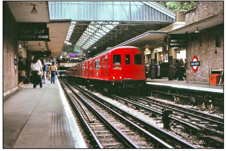
Above: A westbound train stands in platform 3 at Earl's Court on 10 August 1978 destined for Ealing Broadway with a CP Stock motor car leading. By this time, headlight codes on the District had been abolished and trains were required to show just the bottom two lights for any destination.
