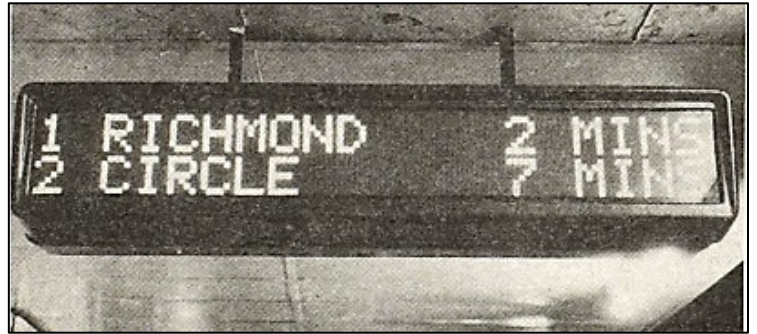
Above: The experimental 1981 dot-matrix indicator at St. James's Park westbound.
