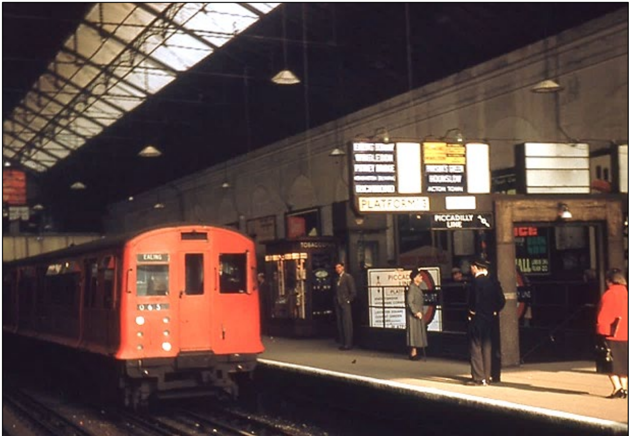
Above: A red-painted R Stock arrives at Earl's Court westbound platform 3 bound for Ealing Broadway in the 1950s. The yellow NOT STOPPING AT plates are clearly visible. Above the staircase is a 'switchable sign' operated by station staff. This advised Olympia passengers to wait for special trains or, if these were not operating, change at West Kensington for bus route 28.
