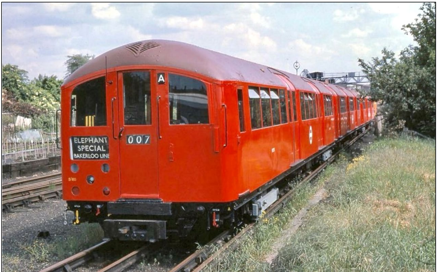
Below: Heavy overhauls and repaints from Acton Works always looked immaculate, as with this 1938 Tube Stock waiting to return to the Bakerloo Line.
