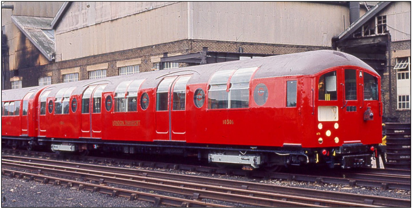
Above: Also looking pristine is the one-off “sunshine window” or “vista dome” car 10306 of 1938 Tube Stock after its overhaul and repaint in Acton Works in 1971.
