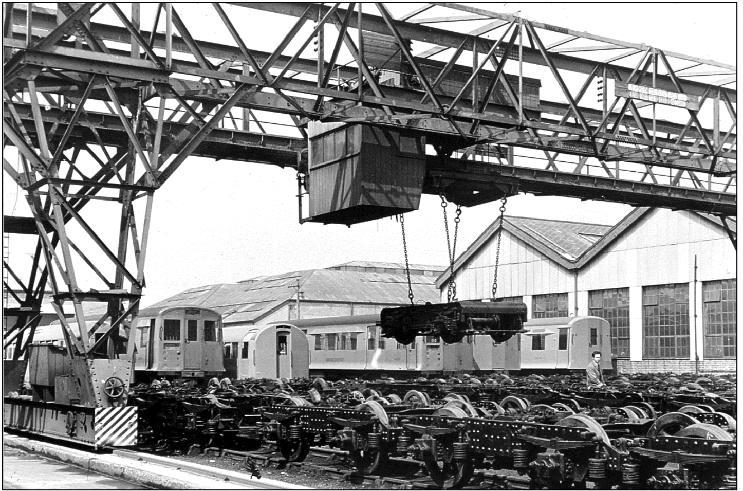
Above: Out in the Works yard, with a line up of freshly overhauled bogies, with one being moved by the overhead crane. Cars of 1938 Tube Stock and P Stock are in evidence.
