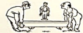
Arrange beforehand which end is to be raised first. Lack of co-operation means crushed fingers.
