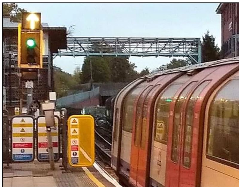
Figure 1: A 1992 Tube Stock train about to depart from the EB platform at Leytonstone, the starting signal showing the 3-aspect signals used to provide proceed indications for both manually driven and automatic trains, like those on the Victoria Line. The Central Line upgrade project of 1990-2005 included the 1992 Tube Stock and new ATC signalling installed by Westinghouse. Note the new style of route indicator introduced on this line with an illuminated arrow indicating each direction rather than three while lights being shown only for diverging routes. The arrow seen here indicates the route straight ahead. Unlike the older route lights, these new indications were not required to be proved. Photo: Phil Wimbush.
