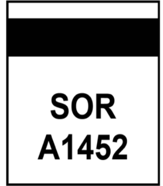
Figure 5 (above right): A signal identification plate for an automatic visual signal on the Central Line. The code letters refer to the area, in this case, South Ruislip. The signal is the westbound home.
