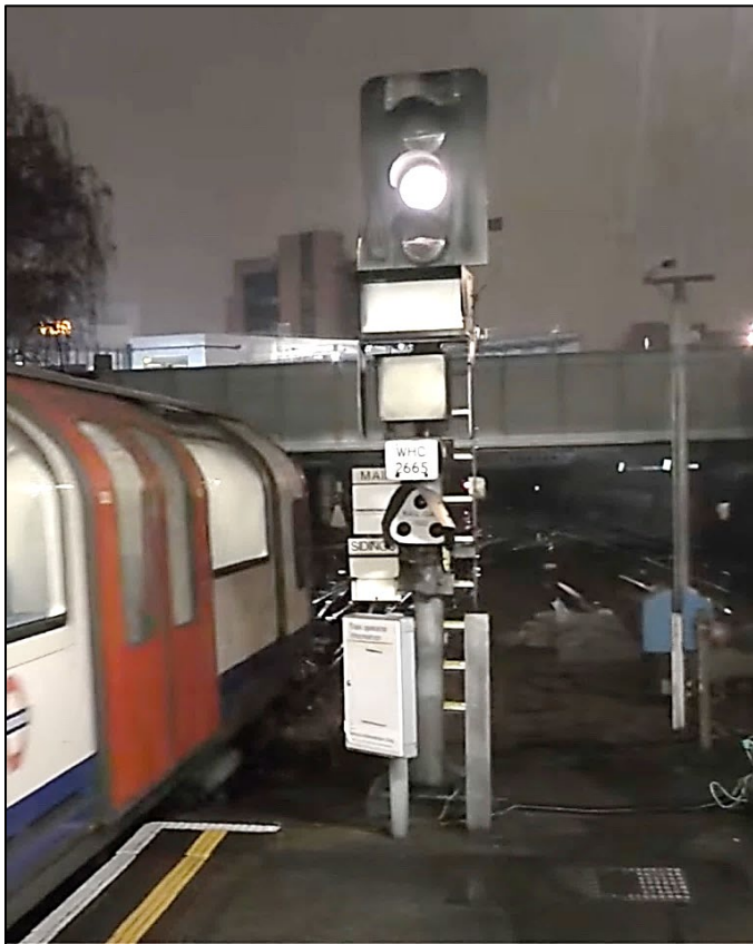
Figure 7: An example of a 3-aspect signal on the Central Line at White City. It has its aspects arranged from the top as Green, White and Red. The white aspect is shown for the departing train, which is in ATO mode. Trains in coded manual are not permitted to pass the signal unless a green aspect is shown. Below the signal is the 'Route Secure' sign and below this is the square sign where a shunt signal is displayed if required. The signal number is on a small rectangular plate, showing WHC 2665. Below that is a triangular rail gap indicator. Photo: Still from YouTube video by x2k9.
