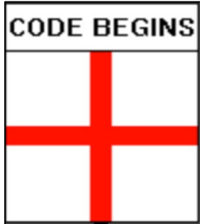
Figure 5 (above right): A signal identification plate for an automatic visual signal on the Central Line. The code letters refer to the area, in this case, South Ruislip. The signal is the westbound home.
