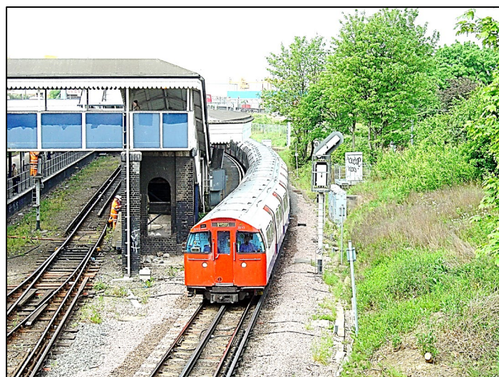
Above: Engineering mods saw the train whistle relocated above the offside cab window as seen on this southbound train at Stonebridge Park (Left), which meant moving the car number at that position, giving an uneven frontal appearance. Note also the front cab door opening handle at the bottom. To the layman, the unique four-car unit 3299 (Right) on the southbound leaving Willesden Junction, looks no different from the rest, but in a train formation it is the only one with two UNDMs in the middle. To the engineers, all four cars were originally opposite facing until converted to this hybrid unit.
