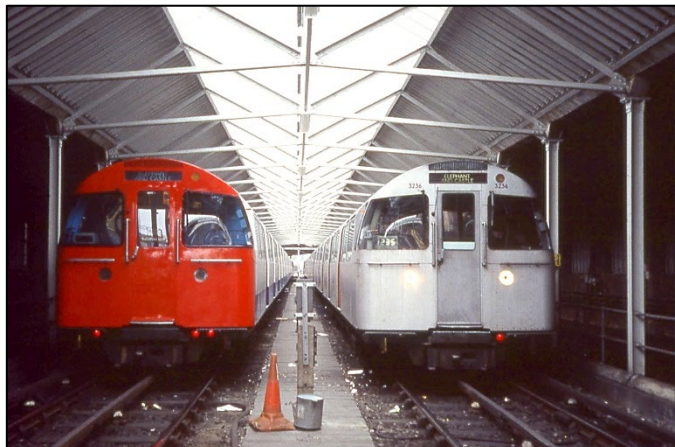
Above: (Left) The refurbished Bakerloo Line trains did not initially have the car numbers re-applied over the cab windows, as seen on a recently refurbished train in the North Shed at Queen's Park, next to an unrefurbished train, this one being sent for refurbishment in June 1994 as Train 27.
