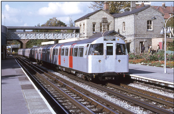
Above: The 1972 MkII Tube Stock first saw service on the Northern Line and an example in fairly new condition is seen arriving at Finchley Central (Left). It is fitted with an electronic destination blind and train set number box (at the bottom of the offside cab window), the latter actually being very difficult to read in daylight. Most trains of 1972 MkII Tube Stock had conventional destination blinds and traditional train set number plates in melamine, as seen at High Barnet (Right).
