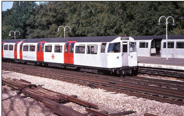
Above: The 1972 MkII Tube Stock first saw service on the Northern Line and an example in fairly new condition is seen arriving at Finchley Central (Left). It is fitted with an electronic destination blind and train set number box (at the bottom of the offside cab window), the latter actually being very difficult to read in daylight. Most trains of 1972 MkII Tube Stock had conventional destination blinds and traditional train set number plates in melamine, as seen at High Barnet (Right).
