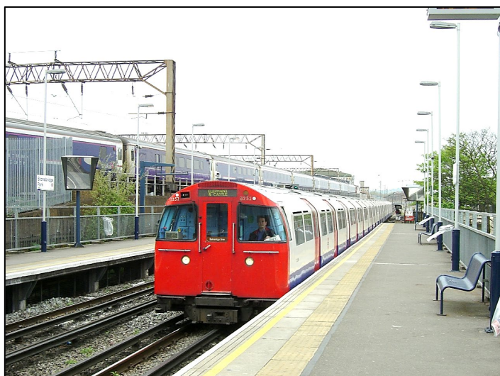
Above: Engineering mods saw the train whistle relocated above the offside cab window as seen on this southbound train at Stonebridge Park (Left), which meant moving the car number at that position, giving an uneven frontal appearance. Note also the front cab door opening handle at the bottom. To the layman, the unique four-car unit 3299 (Right) on the southbound leaving Willesden Junction, looks no different from the rest, but in a train formation it is the only one with two UNDMs in the middle. To the engineers, all four cars were originally opposite facing until converted to this hybrid unit.
