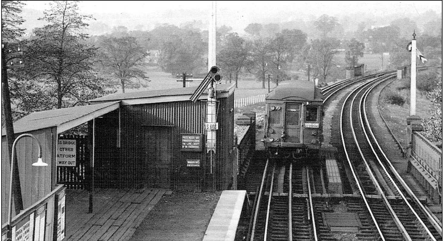
Figure 2: A single, middle motor car train of District 1905 Stock leaving Park Royal & Twyford Abbey, looking west towards South Harrow sometime in the 1920s. The original experimental signalling has been updated. The starting signal has a new semaphore arm and operating cylinder and it shows the white horizontal stripe provided on the arm to denote that it is an automatic signal. Although the train has passed the signal, it still displays a proceed indication because the train is still in the overlap. Modern Underground installations have additional track circuits that cause the signal to return to danger as soon as the front of the train passes it. Note the repeater signal on the other track automatically displaying that the starting signal is off. Photo: Author's collection.
