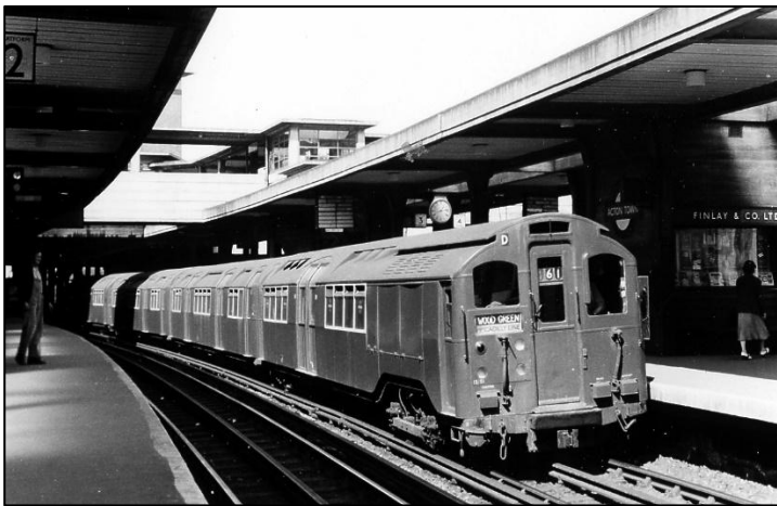
Above: (Left) A four-car train arrives in the eastbound at Acton Town in c.1953 with a 1927 MCCW motor car leading. Note that that the motor car has passenger open door buttons fitted, although such a facility was never introduced on the Piccadilly Line. At this stage, overhauls from Acton still applied cream around the windows. The train set number still has to be relocated in the offside cab window although it does have a proper window wiper.
