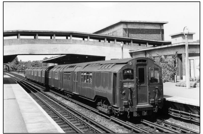
Above: (Left) A four-car train arrives in the eastbound at Acton Town in c.1953 with a 1927 MCCW motor car leading. Note that that the motor car has passenger open door buttons fitted, although such a facility was never introduced on the Piccadilly Line. At this stage, overhauls from Acton still applied cream around the windows. The train set number still has to be relocated in the offside cab window although it does have a proper window wiper.
