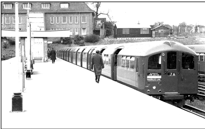
Above: (Left) Stanmore in the early days of Bakerloo Line uncoupling with a four-car train in platform 2 awaiting departure. The heavy overhaul date on the leading motor car is 2/51 and the train appears to be in ex-works condition. To its right is an uncoupled unit stabled in Stanmore Sidings. The destination plates of "Elephant" (over) "and Castle" were later replaced by "Elephant" plates with larger lettering which were easier to read.
