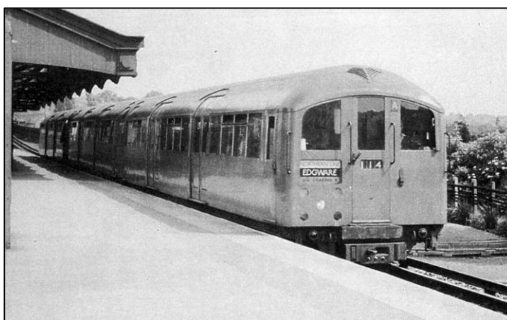
Above: (Right) A three-car unit of 1938 Tube Stock at Brent, working the Kennington – Edgware via Charing Cross route, having been uncoupled from train 14 and now working as train 114. This was one of the three-car units which had two compressors on the trailer car.
