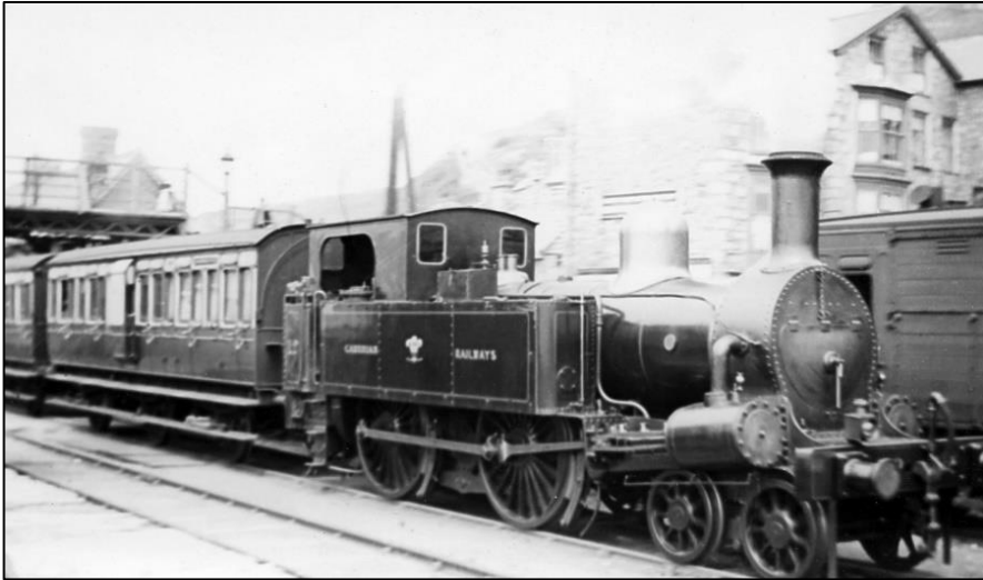
Cambrian Railways Beyer Peacock 4-4-0T number 12 (former Metropolitan Railway number 11 and subsequently GWR number 1130) with a passenger train at an unknown location. Behind the engine is a six wheel passenger brake coach.
