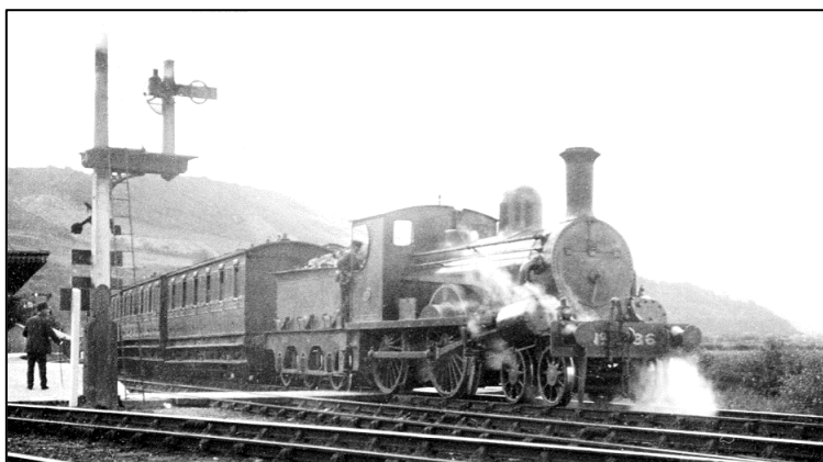
Cambrian Railways Beyer Peacock (426/1864) 4-4-0 number 36 (formerly Met Rly No.15 "Aurora") on a passenger train at Barmouth North junction. Allocated
