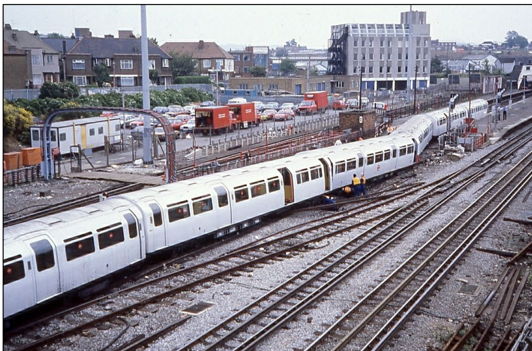
Left: On 20 July 1986, a six-car train of 1983 Tube Stock derailed on the approaching Neasden southbound, three cars coming off the road and causing much track damage. The LT Breakdown gang are seen in attendance with their red vehicles in the background. The two units involved were 3615 and 3629 which did receive an overhaul at Neasden and Acton Works respectively. A similar derailment occurred in the same location on 14 August 1989
