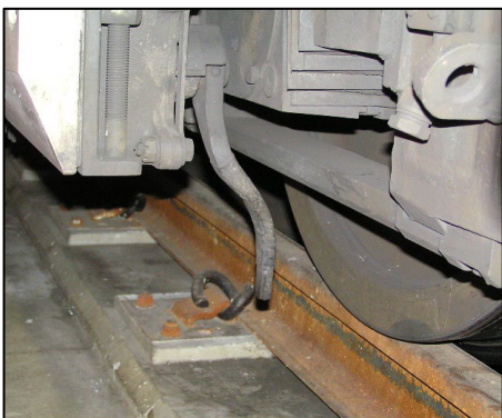
Tripcock arm on 1995 Tube Stock, Northern Line, in the set position.
