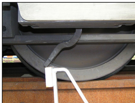
1995 Tube Stock in Golders Green Depot in the process of being tripped, for demonstration purposes, on a specially installed fixed trainstop.
