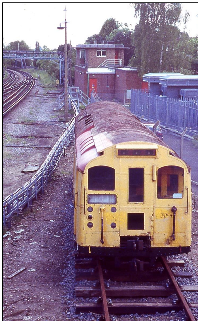
Above: Two views of L11 shunting in Acton Works, the top photo showing its original service stock 'maroon' livery with the two couplers visible and then after repainting in yellow livery. The west end did not have two couplers as this would be unlikely to be used often in shunting stock in Acton. On the right is L11 after arrival at Epping but before any restoration work had begun on the locomotive and in the signal cabin.
