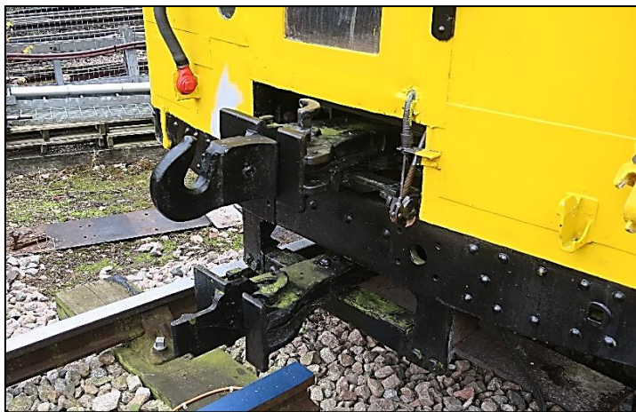
Above: (Left) A close up of the two separate but fixed couplers that was provided at one end of L11 which, for a time, complemented the original Acton Works shunter (L10 – which was scrapped in 1978), which had adjustable couplers at both ends.
