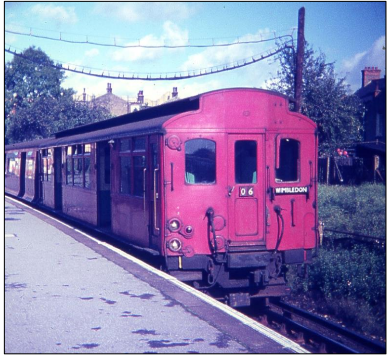
Above: Q23 motor car 4200 leads a mixed formation Q Stock on the westbound at Wimbledon Park. This was one of the cars that was part of the centre-guard experiment in 1948 and was also fitted with outside door indicator lights, the diamond housing still being visible but not in use.
