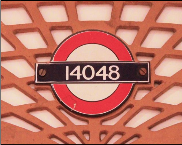
Above: Examples of restored interior car number plates. That (Left) is from an O Stock mounted on the wing-shaped grille (note, number not in Johnston font), while those (Right) are from P Stock. 13257 and 14217 would have had '5' replace the first '1' on PCM conversion but 014271 was converted to a motor car in 1949 and became 14271 and then latterly 54271.
