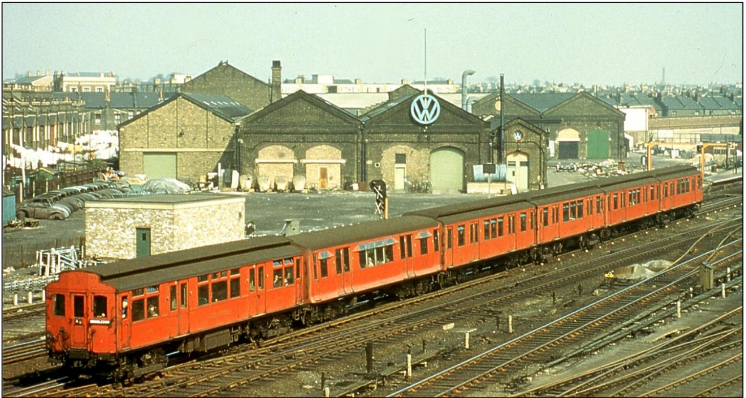
Above: This photo of a six-car mixed Q Stock train leaving Plaistow shows the varying design styles this group of stock embraced. On the left is a Q23 motor car (known as 'horse boxes') and to the right a Q38 trailer, just 15 years younger – how the designs changed. Next is a Q31 or Q35 trailer, a Q27 motor car, another Q31/35 trailer, and a Q27 motor car bringing up the rear. Above the second car can be seen an LT-style signal but not yet commissioned (having white crosses on them), which dates prior to the October 1959 resignalling and BR/LT track segregation.
