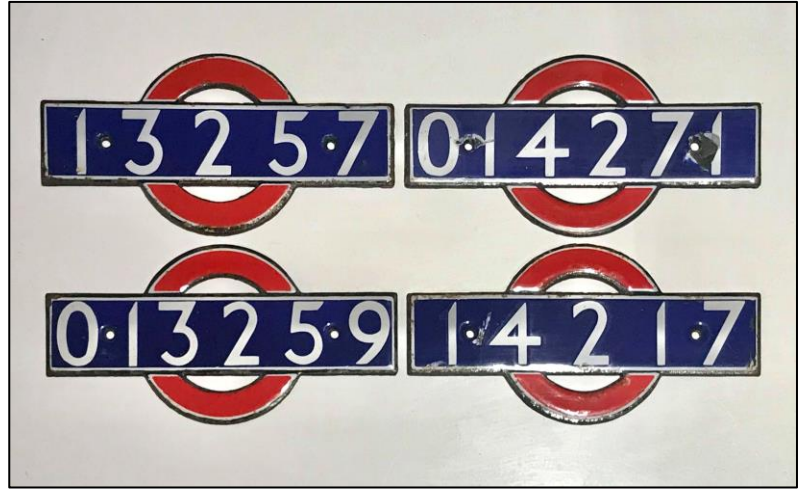
Above: Examples of restored interior car number plates. That (Left) is from an O Stock mounted on the wing-shaped grille (note, number not in Johnston font), while those (Right) are from P Stock. 13257 and 14217 would have had '5' replace the first '1' on PCM conversion but 014271 was converted to a motor car in 1949 and became 14271 and then latterly 54271.
